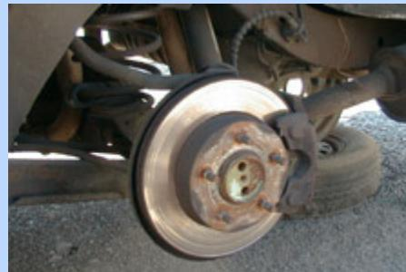
To our surprise, we found that Lincoln used four-wheel disc brakes on some Mark series cars during the 70's. We contemplated fitting the rear disc setup on the Gran Torino.
