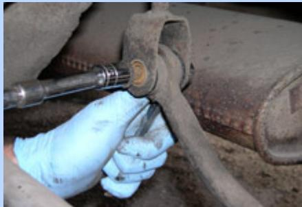
**5** We removed the upper control arm-to-housing bolts. In hindsight, removing the trailing arm-to-housing bolts first would have been a better route. Regardless, we unbolted both, kept the hardware and kept moving.
