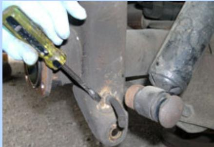
**4** No jacks allowed at this wrecking yard, we threw a tire under the pumpkin for support. Since we had already tossed the calipers and rotors we went ahead and pulled the axles so we could manage the housing. Yes, we kept the axles! Once the shock was unbolted, we popped out the parking brake cable.
