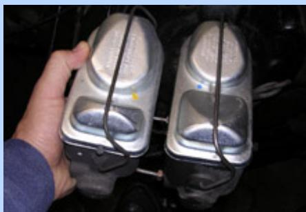
**11** To accommodate the rear discs we also needed the master cylinder out of the Lincoln. We chose to go ahead and buy a remanufactured unit from the parts store rather than take the time to pull the used piece. Take note of the larger rear brake reservoir used on the Lincoln master cylinder (right).
