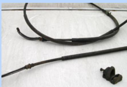
**13** Finally, we took both parking brake cables. We later found that we actually needed two of the shorter (lower in photo) cables to make it work. We did not need the longer cable shown tied in a loop at the top of the photo.
