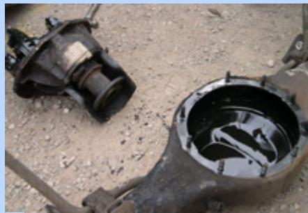
**10** We were planning to reuse the original 3.25:1 dropout from the Gran Torino so we left the 2.50:1 Lincoln dropout behind.
