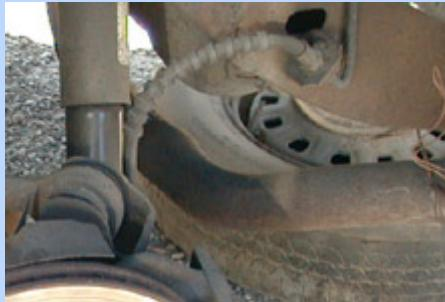
**3** We did not toss the flexible brake hoses, they were both in good shape. These lines run about \$35.00 each at the parts store. We also took the brackets which secure the brake lines to the frame.
