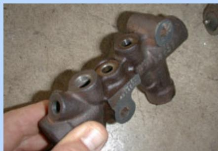
**12** The Gran Torino proportioning valve would not be correct for the new disc brake rear either. We grabbed this valve out of the Lincoln. They are noticeably different. Mistakingly, we assumed the Torino master cylinder-to-proportioning valve lines would be the same. They were not. We cut the Lincoln lines to get to this valve out. Doh! Luckily there was another Lincoln in the yard with similar lines.
