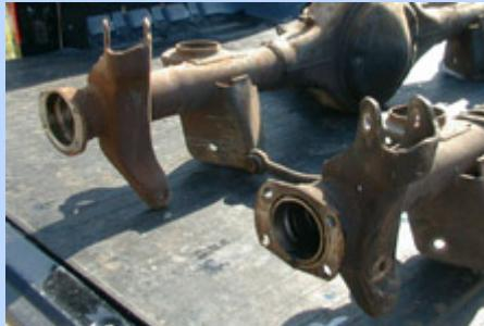
**3** Side by side, we could see there was very little difference between housings. However, the Lincoln Housing (close) uses a larger axle flange with a wider bolt pattern than the Gran Torino housing (far). The bearing bores are also different. The Lincoln housing also has a thru-hole for the parking brake cable.
