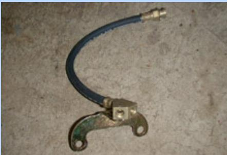
**9** The junction/flexible brake hose we used here is not required for the Lincoln since its' rear brake lines run along the frame rail. However, the rear brake lines on the Torino run from the hose to hard lines that run along the axle. The hose was unusually expensive for what we got. About \$40.
