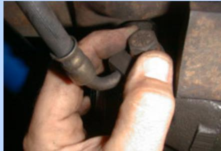
**8** We installed the flexible brake hoses that we picked up at the salvage yard.
