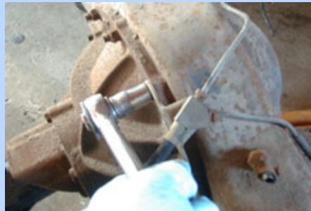
**2** We wanted to use the 3.25:1 third member from the Gran Torino so we pulled that before we ditched the housing. Both cars used 28 spline axles. We considered keeping the combination junction/flexible brake hose, but it was brittle. We discarded hard brake lines since we'd be making new ones.
