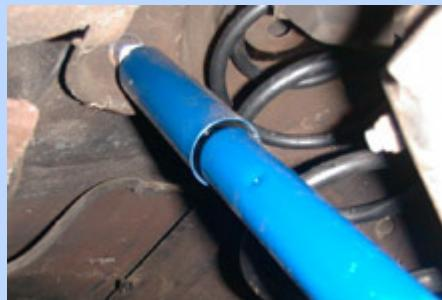
**6** We installed the rear shocks. The mounting point on the axle housing was
