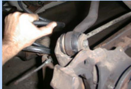
**4** The Lincoln rear-end was now complete with our original third member and reinstalled Lincoln axles. We slipped the unit under the car with a floor jack and attached the upper control arms. We were eager to test fit the springs in order to confirm the perches were the same. As we hoped, they were.
