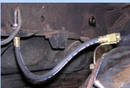
**11** We attached the flexible brake hose to the hard line mounted to the underside of the tub.
