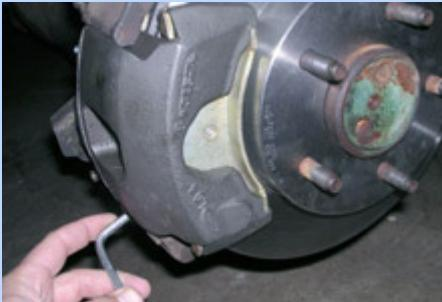
**7** We installed new calipers and rotors. We picked up these rotors from Napa for about \$30 a piece. After some shopping around we found these "unloaded" A1 Cardone rebuilt calipers for \$49 each and pads for both left and right were \$19. Don't be fooled, the same caliper was being sold "loaded" for \$90 each at most automotive parts chain stores.
