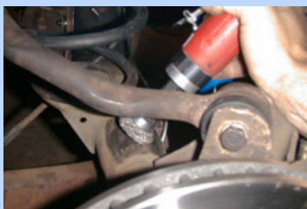
**15** We cleaned up the axle housing where we intended to weld the bracket.
