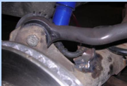
**17** Secure the flexible brake lines to the newly attached brackets. We chose this location because it gave the line a good buffer between moving parts.
