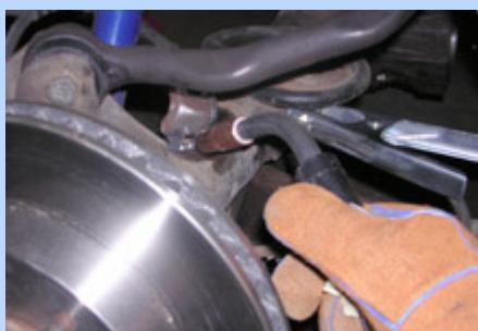
**16** We cleaned up a nice spot under the spring perch for good connectivity. Next, we taped down the bracket so it would rest flush against the housing for a good weld.
