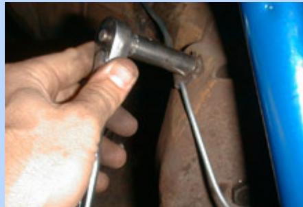
**20** We secured the hardlines with the mounting hardware pulled from the original Gran Torino axle housing.
