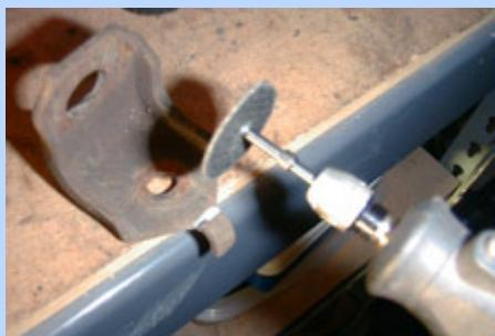
**13** This is one of the flexible brake line-to-frame brackets we pulled from the Lincoln. We decided to reuse it by welding it to the axle housing, but first we needed to remove the location tabs.
