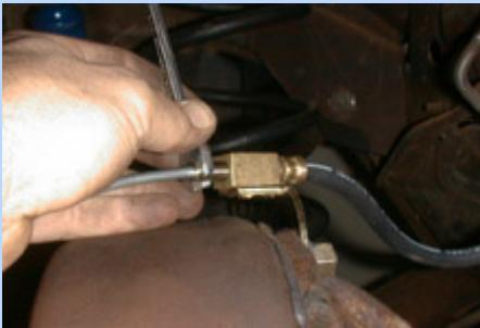
**19** With the hard lines bent correctly, we connected them to the junction/flexible brake hose.
