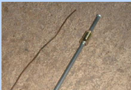
**18** With all three of our flexible brake lines mounted we could install our hard lines to run along the axle. We bought (2) 30" lines from the parts store and templated the bends with a piece of bailing wire.
