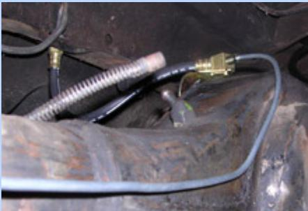
**21** The Lincoln rear-end with disc brakes was now installed and plumbed. It was time to move to the motor compartment to install the Lincoln master cylinder and proportioning valve.
