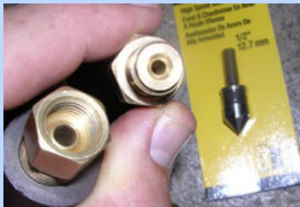
**23** This modification lives up to FordMuscle's promise to bring you the real story when performing upgrades. The original Gran Torino hard line (running to rear junction/flexible brake line) would not fit the female thread on the proportioning valve. We hunted high and low for the right fitting. In combination, these two did
