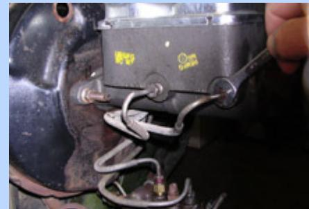
**25** We bench bled the master cylinder and installed it. Following that we installed the hard lines connecting it to the proportioning valve.
