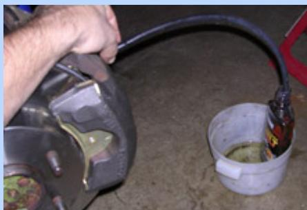
**26** The system was now ready to be pressurized. We bled the brakes and found no leaks. We had a firm pedal but no power to road-test the car. The '73 Gran Torino factory 429 car is awaiting a drivetrain.
