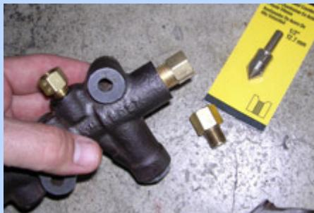
**22** We needed three fittings and a counterbore to make the Lincoln proportioning valve work on the Gran Torino. If we had used the donor car master cylinder-to-proportioning valve lines we would not need the leftmost fitting shown in the picture.
