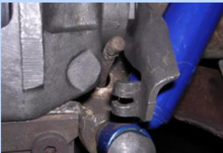
**9** We threaded the caliper end of the parking brake cables through holes on the shock mounting brackets.
