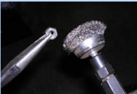
**5** Obviously, cutting down the cables meant we would lose the ferrules. We opted for the quick and dirty route. This nut was about the same diameter as the ferrule. We planned to simply weld one to each cable after giving them a quick wire brushing.
