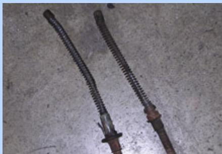
**2** The cable on the left is one of the Gran Torino cables, it is meant to mount to the drum backing plate. The Lincoln cable mounts to the axle housing just above the shock. Even though they were nearly the same length, the Gran Torino cable would not work.
