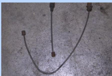
**3** The shorter Lincoln cables were still a little long to fit the intermediate frame of the Gran Torino. Again, the Gran Torino cable is shown on the left. With a little modification to two short Lincoln cables we made them fit.
