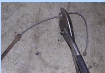
**4** We cut down both the short Lincoln cables to match the length of the original Gran Torino cables.
