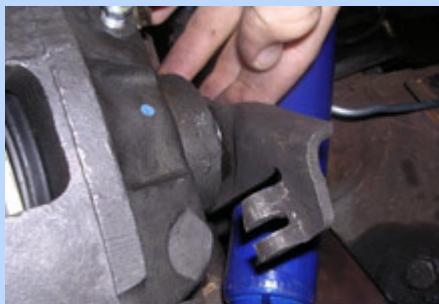
**8** We attached the parking brake cable brackets to the back each caliper. This is a view of the rear driver side caliper. We had pulled the brackets from the original calipers we ditched at the salvage yard.
