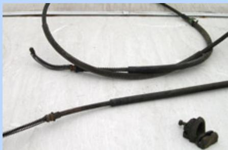
**1** The Lincoln had different size cables running to each caliper. One long and one short. The Gran Torino was set up with two equal size cables. The shorter Lincoln cable was almost the same length as each of the Gran Torino cables. We needed an additional short cable from another Mark series car with disc brakes. Fortunately, there were two in the yard so we acquired the second cable.
