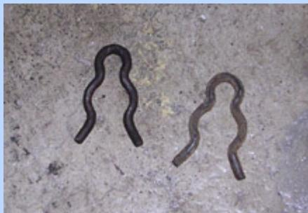
**10** More hardware we were sure to keep from our original salvage yard trip. These clips secure the parking brake cable to the frame and shock mounting bracket. We needed a total of four, two for each cable.
